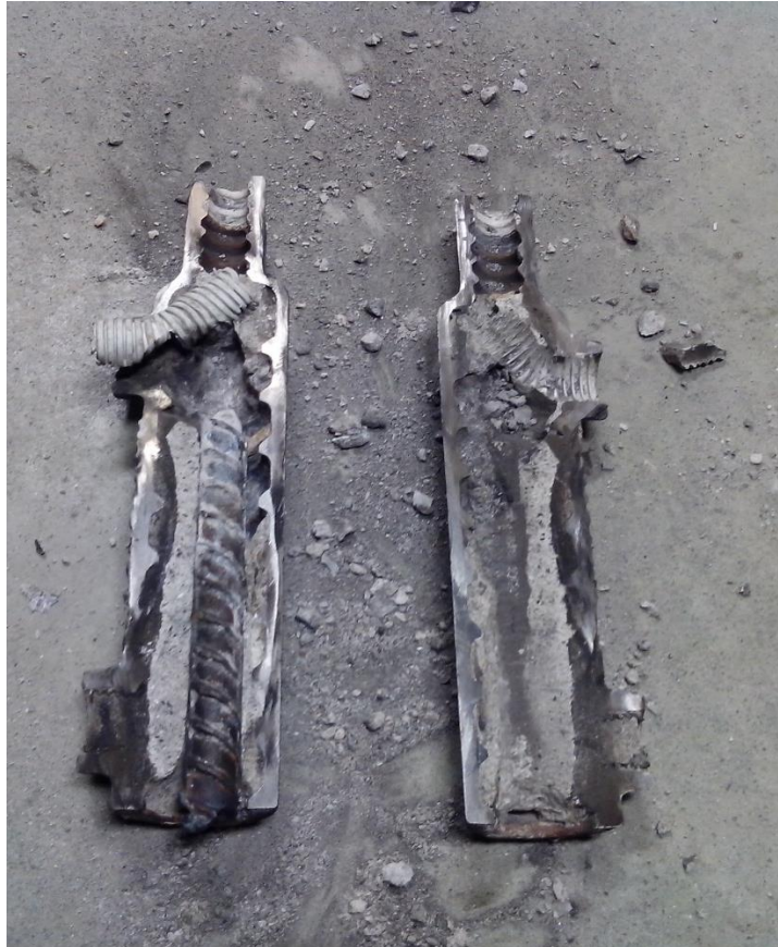
Figure 5: Example photograph of grout sleeve with a short starter bar and voids within the grout
