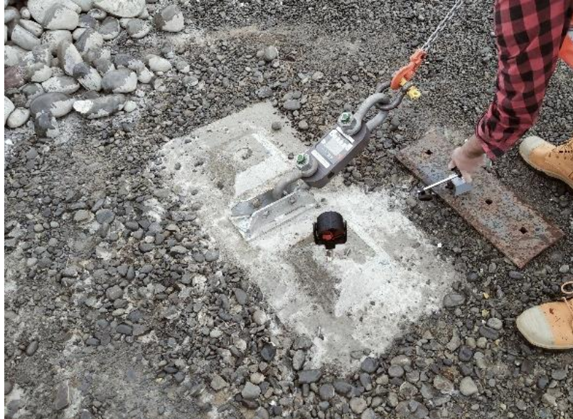
Figure 1: Testing arrangement of concrete ballast test
